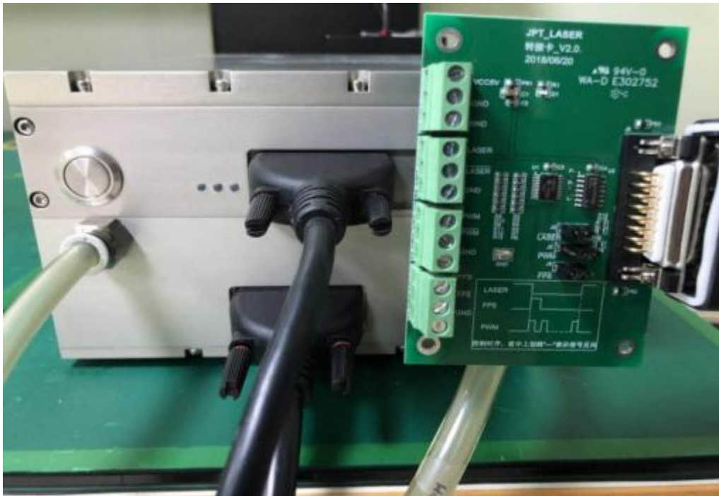
Figure 6 Control signal and adapter card connection
