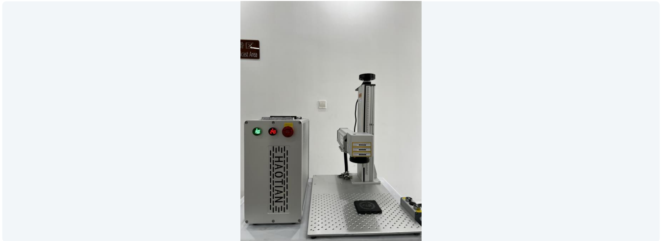
Representative split machine: separate control cabinet, Z tower, scan head and worktable.
